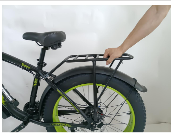
Fix rear fender and rear rack to the frame
