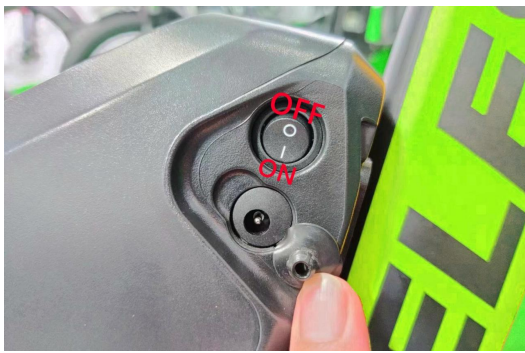
The charging port and the battery ON-OFF switch
