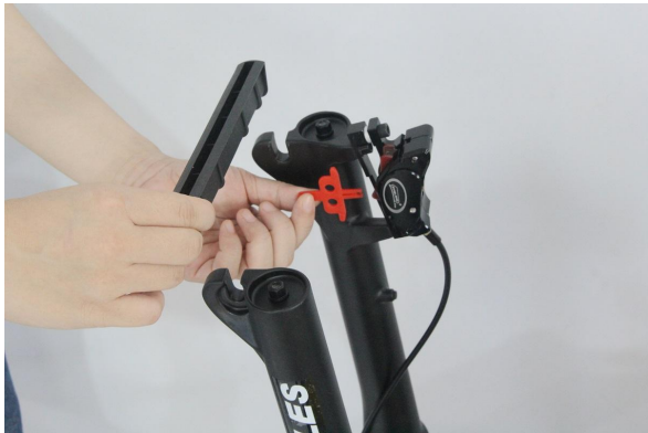
Remove the fork spacer. ( it is not a part of the bike )
