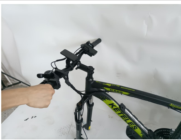
Fit the stem and handlebar together
