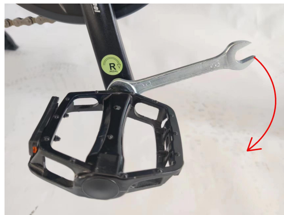
Turn the spanner clockwise to fix the pedal R
