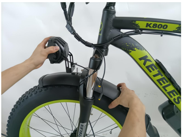
Fix Headlight and fender to the fork brace
